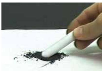
A magnet (the white bar) is brought near the iron sulfide.
