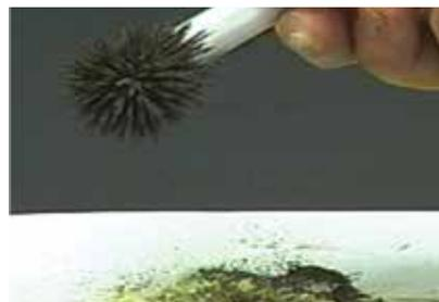
The magnet pulls the iron out of the mixture and leaves the sulfur behind.
