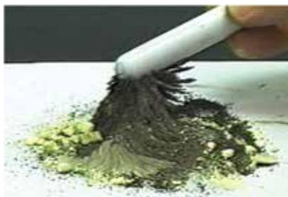
A magnet (the white bar) is brought near the mixture.
