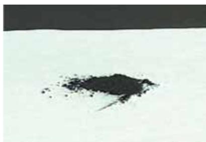
Sulfur and iron are mixed together and then heated so that they form the compound iron sulfide (the black powder).
