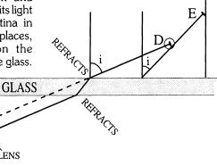
4a. Ray C has the same angle of incidence as ray D. (Pins A
