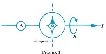
The magnetic field B will form as indicated by the compass needle's direction. The needle aligns with the magnetic field.
